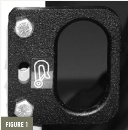
Crash tested securement point labeled with hook symbol
