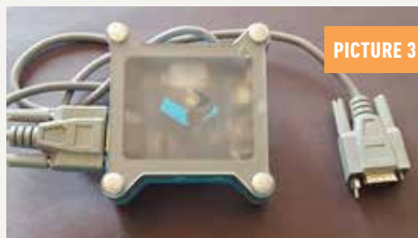
The Tecla Shield connects to the power wheelchair through the Auxiliary module. Once connected, users follow a series of steps to pair the device with a Bluetooth capable phone.
