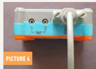
The Tecla Shield connects to the power wheelchair through the Auxiliary module. Once connected, users follow a series of steps to pair the device with a Bluetooth capable phone.
